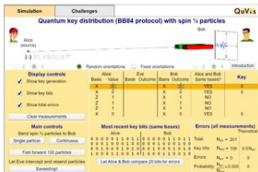
Figure 8. BB84 Simulation with \frac{1}{2} spin particles –no interception, random selection of the measurement bases (orientation)
