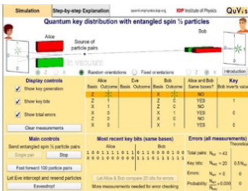
Figure 15. Simulation BBM92 – no interception, random selection of the bases/alignment axes/ particles deflection
