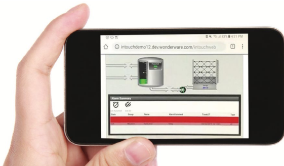
Fig. 7: . Representation of the HMI simulator which was accessed remotely using the mobile device (Software used: Aveva InTouch HMI) https://www.aveva.com/en/solutions/operations/operations-control-hmi/
