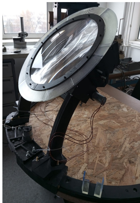
Figure 1. Experimental model of the sun tracking system for the planar concentrator
